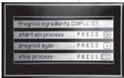
Fig. 3-8: After finishing the pregrind program
